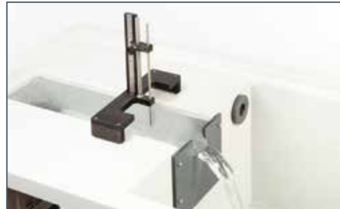
Sharp-crested overfall at a measuring weir
