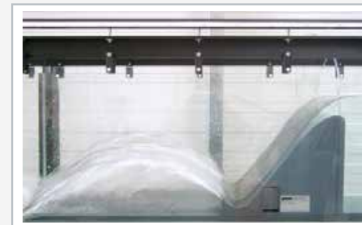
Overfall at the ogee-crested weir with ski-jump weir outlet HM 163.32.
