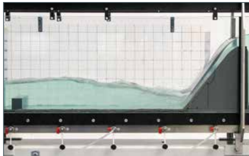
Ogee-crested weir with a sill
