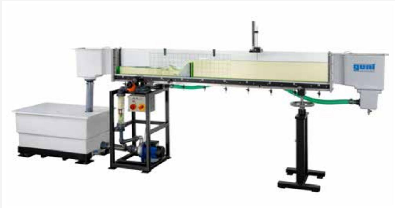
The illustration shows HM 160 together with the ogee-crested weir HM 160.32 and the level gauge HM 160.52.
