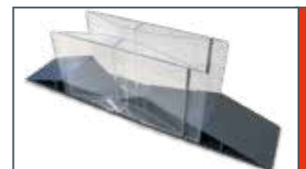
HM 162.55 Parshall flume
