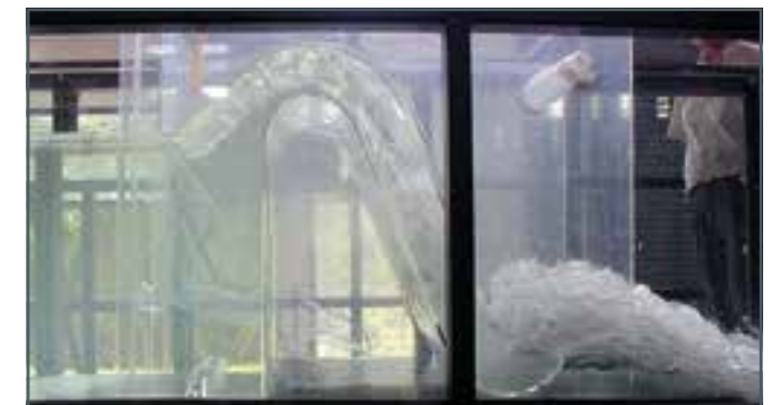
Discharge in the active siphon weir HM 161.36
