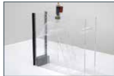
Siphon weir HM 160.36
