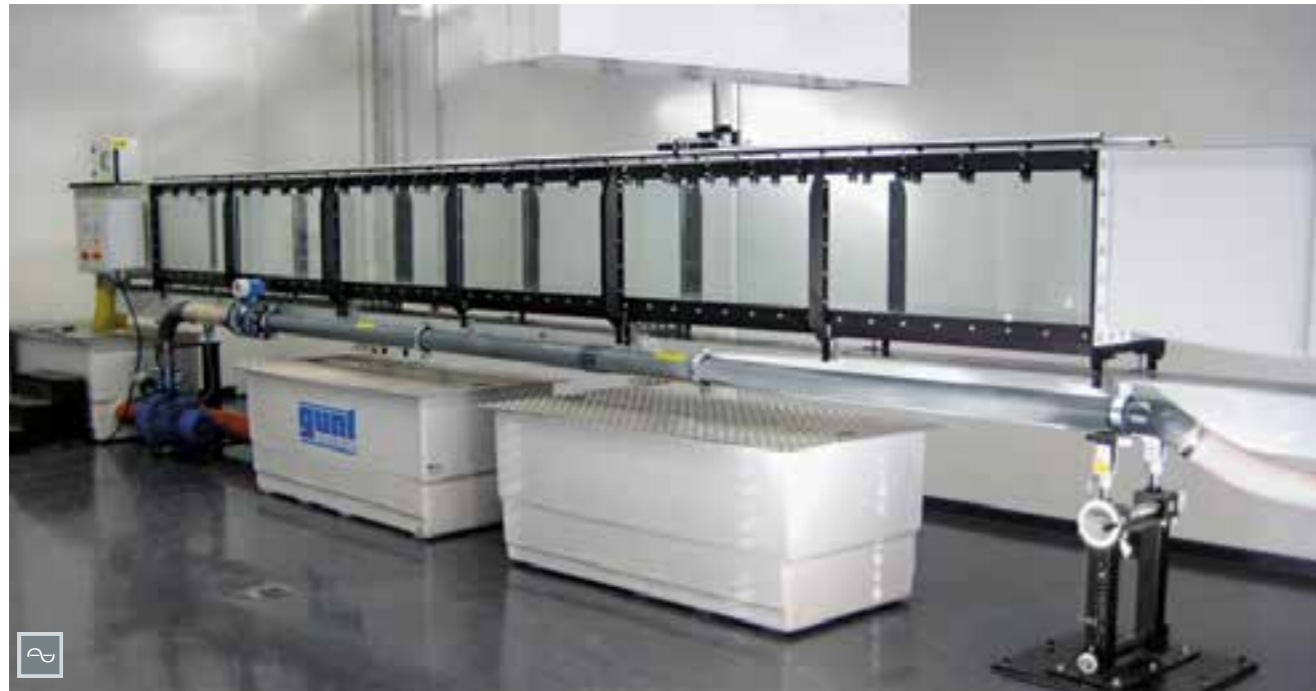
The illustration shows HM 162 (7,5m experimental section) with the wave generator HM 162.41 and the level gauge HM 162.52.
