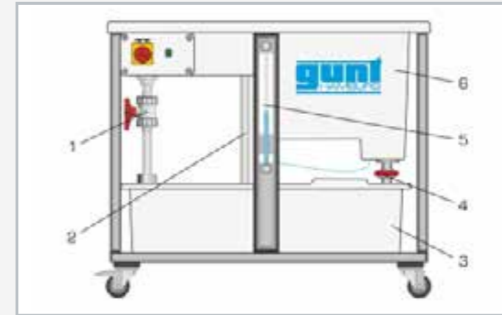
1 flow control valve, 2 overflow, 3 storage tank with submersible pump, 4 gate valve for emptying the measuring tank, 5 measuring tank level indicator, 6 measuring tank
