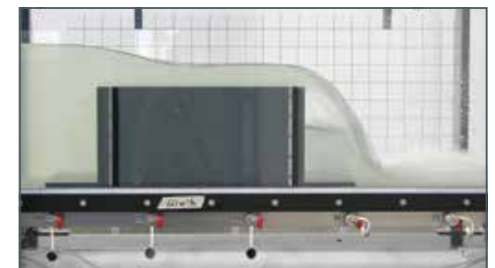
Broad-crested weir HM 162.31
