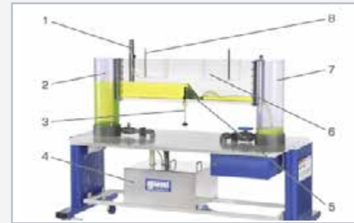
1 sluice gate, 2 water supply, 3 sill height adjustment, 4 supply tank, 5 ogee-crested weir used in the experimental flume, 6 upper limit, 7 water drain with plate weir at the water outlet, 8 measuring tube
