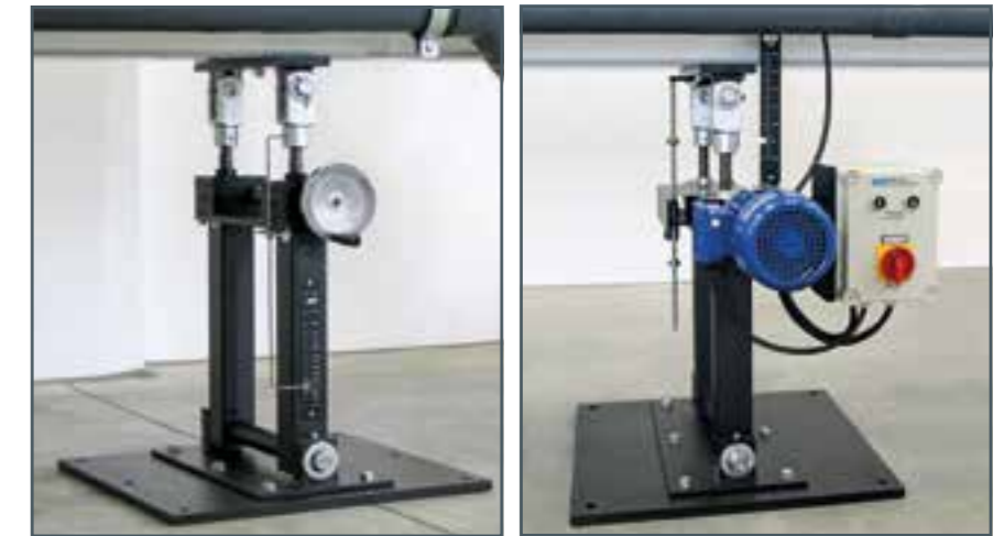
Inclination adjustment in HM 162 and HM 163: left manual, right electrical inclination adjustment HM 162.57 / HM 163.57
