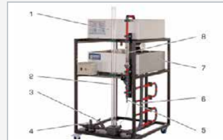
1 basin A with adjustable weir, 2 surge chamber, 3 valve in drain pipe, 4 gate for generating water hammer, 5 water connection, 6 overflow pipe, 7 basin B with overflow, 8 flow meter
