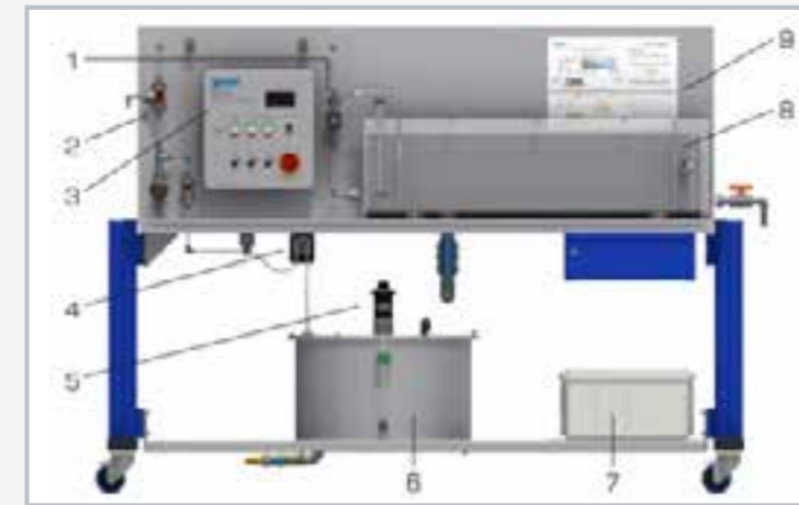
1 electromagnetic flow rate sensor, 2 sampling point, 3 switch box, 4 pump, 5 stirring machine, 6 suspension tank, 7 storage bin, 8 sedimentation tank, 9 illumination
