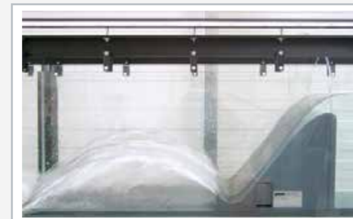
Overflow at ogee-crested weir with ski jump spillway HM 162.32.
