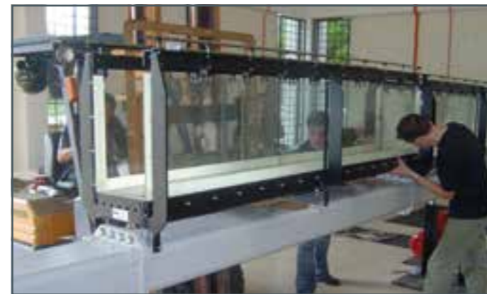
The experimental section element is placed on the carrier with a forklift, aligned and installed.
